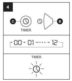
5. To set the timer power on, while powering off the unit press the Timer button on the control panel (C).
