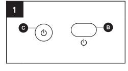
Select a heat setting by pressing the HEAT button on either the control panel (C) or the remote control (B) to toggle between the three heat settings.
