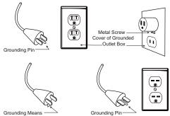
**A WARNING:** It is normal for the power cord to feel warm to the touch. However, a loose fit between the outlet and the plug may cause overheating of the plug. If this occurs, try inserting the plug into a different outlet. Contact a qualified electrician to inspect the original outlet for damage.
