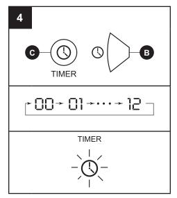
To set the timer power on, while powering off the unit press the Timer button on the control panel (C).
