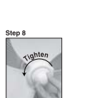
Step 8 Thread Blade Cap onto threaded end of Motor Shaft. Note: Threads are reversed. Tighten = Counter-clockwise.
