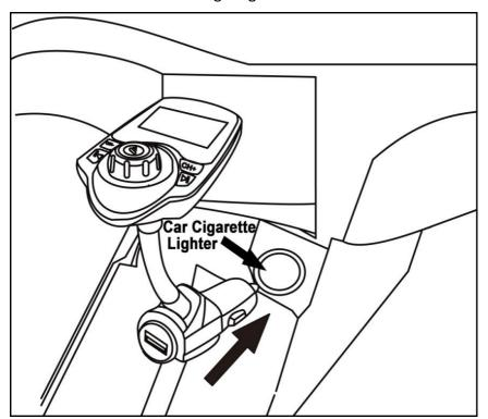
2. The unit will automatically power on and the voltage of the car battery will appear on the LCD Display on the unit as illustrated below:
