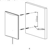
3. Insert the supplied plastic inserts into the holes by hammer (Not Supplied).
