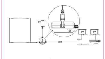
4. Connect the AC/DC Adapter to wall outlet having AC 110-120V, 60Hz as is illustrated below, the power on indicator on the Detachable Amplifier and the Main Unit will illuminate.
